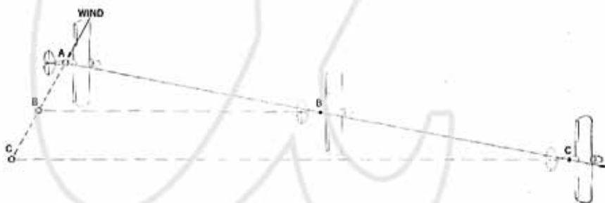
Figure 10.—Airplane and balloon in a wind. ♣
