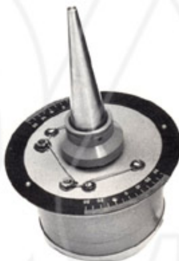
Transmitter/probe is primary sensing unit of AOA system.
