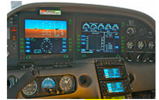
Mark Korin of Alpha Systems believes that his company's angle-of-attack indicators, seen here installed on a Cirrus SR22, can help to reduce the incidence of stall-spin accidents.
