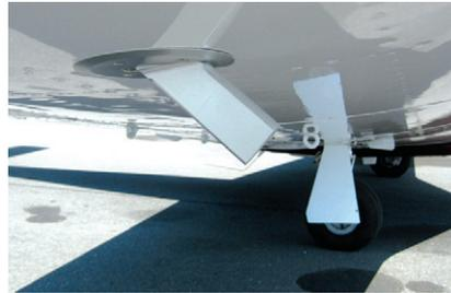
The AOA's probe must be located in undisturbed air clear of the prop blast.
