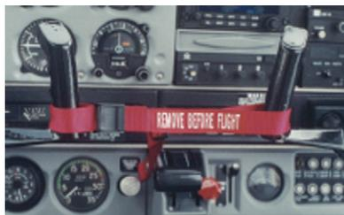
**Piper control lock Holds the Ailerons neutral and the Stabilizer down. Only \$39.95**
