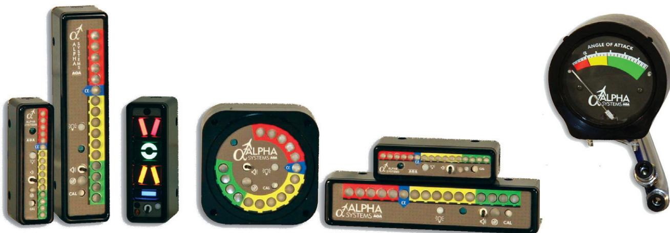
There are six electronic models that offer displays for a panel-mounted dial, vertical and horizontal light bars (two sizes), and the Legacy model.
