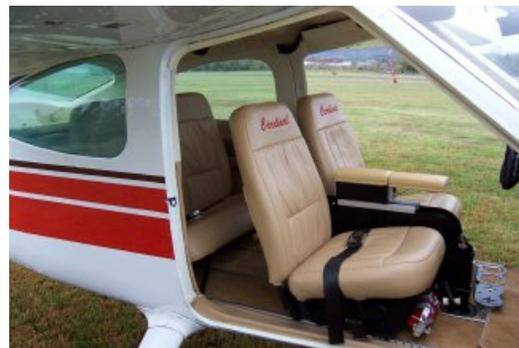
*The Cardinal has the largest interior of any four-place Cessna, which has caused pilots to overload the airplane.*
