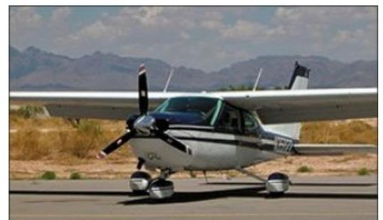
*A three-blade prop looks sharp on a Cardinal. While it reduces vibration and provides more clearance between the tips and the ground over a two-blade, there's no performance increase.*
