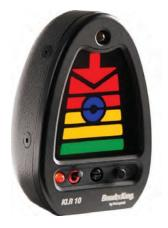
entered the market with its KLR 10 Lift Reserve Indicator this past year. Both sets of systems provide visual and audible indications that are calibrated to the aircraft to provide the pilot a margin of safety before the wing stalls. In fact, the indications will provide the operator the real time dynamic level of the decay in lift as opposed to an airspeed indicator's arbitrary Vso or Vs1 arc indications based on an aircraft's wing design and configuration.
